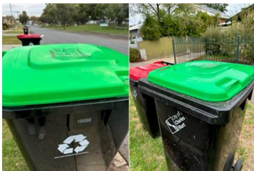
Figure 1: 100% recycled content organic MGBs. Note visual defect with dent in lid
